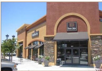
Examples of appropriate window treatments, changes in material and colors to identify entries and storefronts, and use of awnings to frame a window bay or entrance.
